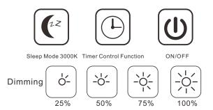
ON/OFF: After the desk lamp is connected to the adapter power supply, the indicator light is red. When the desk lamp is turned on, the red indicator light goes out. The initial on-lamp defaults to 5000K, 75% brightness mode. At this point touch other keys, the mode changes with the corresponding function of the touch key.
